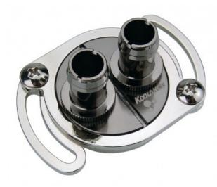
The CHC-122 has improved heat transfer over the earlier CHC-120. It is designed to provide high efficiency liquid cooling for motherboard northbridge chipsets. Versatile mounting hardware allows the CHC-122 to cool almost all types of mainboards, or heat sources up to approximately 175W. Materials include a solid high-density copper cold plate, brass top, and anti-corrosive nickel plating. G 1/4 BSPP fitting threading.
