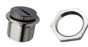
Coolant fill port for configurations without reservoirs (T-line air bleeding), or for separately locating the fill port from the reservoir. Can also be used as a drain valve if positioned low in the system. G 1/4 BSPP fitting threading, with bore size of 18mm (0.7"). Nickle-plated brass.
