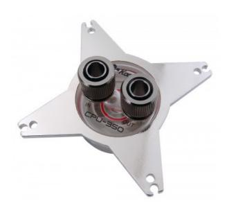
The high pressure CPU-350 is designed for loops dedicated to obtaining the lowest possible processor temperatures. It performs best in systems with a strong pump and few water blocks. Materials include a high-density solid copper cold plate, anti-corrosive nickel plating, and a transparent acrylic (model CPU-350AC) or opaque acetal (model CPU-350AT) top.
