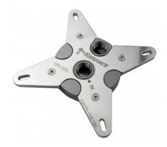
The CPU-370 contains an advanced microfin cold plate (0.25mm fins, 0.30mm channels), o-ring sealed impingement plate, and an optimized flow path minimize coolant restriction.
