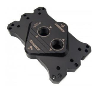
CPU-370SA is a lighter weight, lower priced version of Koolance's acclaimed CPU-370 water block. It includes a similar nickel-plated copper microfin cold plate (0.25mm fins, 0.30mm channels), o-ring sealed impingement plate, and a solid acetal top designed for AMD sockets.
