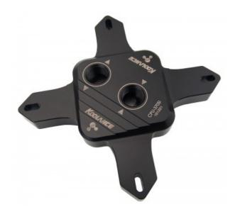
CPU-370SI is a lighter weight, lower priced version of Koolance's acclaimed CPU-370 water block. It includes a similar nickel-plated copper microfin cold plate (0.25mm fins, 0.30mm channels), o-ring sealed impingement plate, and a solid acetal top designed for Intel sockets.
