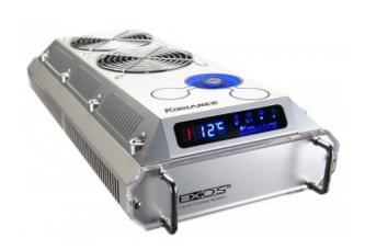
The Exos-2 returns with significantly improved flow rate and control features. "V2" adds a 7L/min (1.85 gal/min), 2.6m (8.5ft) head pump, pump speed control, and rear G 1/4in fitting sockets.
