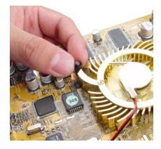
Once loosened, remove the original heat sink. Apply a thin layer of thermal interface compound onto the chipset if necessary.
