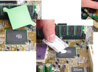
Once loosened, remove the original heat sink. Apply a thin layer of thermal interface compound onto the chipset if necessary.
