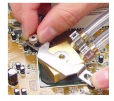
Use the metal attachment nuts to fasten the mounting bracket chipset to the motherboard. Hand-tighten all motherboard components.
