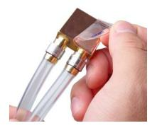
Remove the protective tape from the bottom of the chipset cooler.
