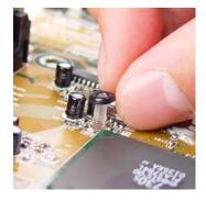
To help keep them secure, place rubber washers over the plastic screws from above the board.
