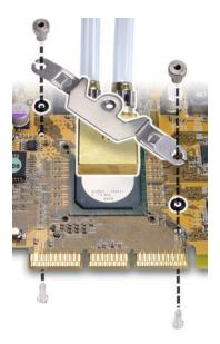
Use the metal attachment nuts to fasten the mounting bracket to the video card chipset. Hand-tighten all video card components.
