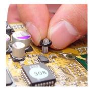
To help keep them secure, place rubber washers on the plastic screws above the board.
