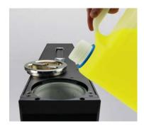
Slowly fill the system with coolant. To maintain the product warranty, use only Koolance approved coolant. Many alternative liquids and additives can cause permanent damage to the cooling unit (through chemical reaction, corrosion, biological growth, high thermal expansion, viscosity, etc.).
