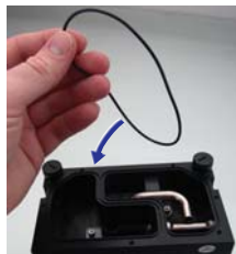
If original o-rings have come out, use the new ones.
