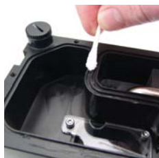
Apply oil to o-ring grooves with a cotton swab.
