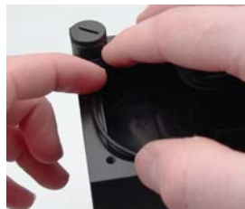
Carefully push an o-ring into the groove around each reservoir.
