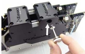
The included long plug is only used for serial flow. Carefully insert this into the right side bridge block as shown.
