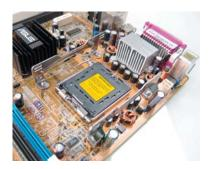
INCORRECT: rails perpendicular to socket locking arm
