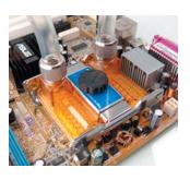
Check that the bracket clips are aligned in all 4 rail holes before installing the tension screw.
