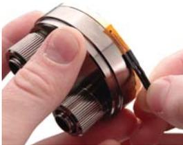
Place the temperature sensor on or near the edge of the gold block. We recommend placing it on the edge. The sensor is required for proper fan speed control and system safety features.
