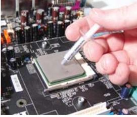
Apply thermal paste to the CPU directly. Spread the paste so that it evenly covers the CPU. A piece of thick paper (such as a business card) works well for this.
