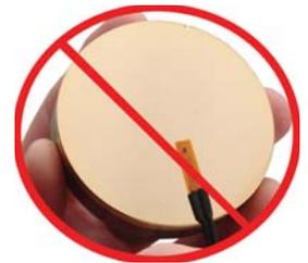
Apply metal tape to keep the temperature probe in place. **DO NOT** stick metal tape or the temperature probe where the processor comes in contact with the cooler.
