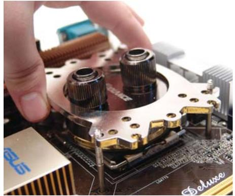
Use either 2 or 4 springs and thumb nuts (depending on socket type) to secure the cooler against the processor.
