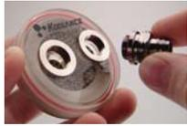
Install two G 1/4" threaded nozzles (sold separately) into the cooling block. Hand tighten all nozzles-- overtightening can damage the block.
