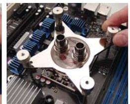
Tighten spring and thumb nuts
