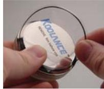
DO NOT attempt to install the temperature probe in between the processor and cooler. Despite its thin size, it will interfere with CPU contact or burn-out the sensor.
