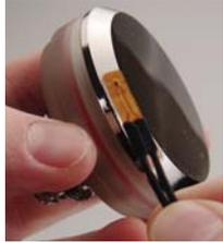
Remove any protective film from the bottom of the cold plate.
