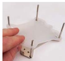
Place the required rubber insulation pad over the bracket posts.
