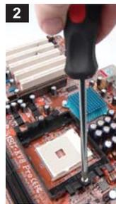
Some processors, like AMD socket 754/939/940, require removal of the motherboard's black plastic retention frame in order to install the Koolance water block.
