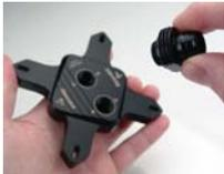
Install two G 1/4 BSP threaded nozzles (sold separately) into the cooling block. Hand tighten all nozzles-- overtightening can damage the block and threads.
