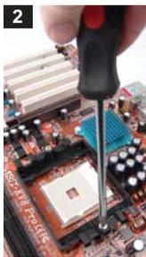
(CPU-370SA only) Some processors, like AMD sockets AM2/AM2+/AM3, may require removal of the motherboard's existing retention frame in order to install the Koolance water block.
