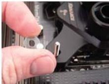
Install the optional plastic washers over each post. These help protect the CPU block from getting scratched.
