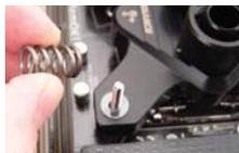
Place the tension springs onto each post.
