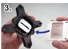
3. The cold plate microfins must run **perpendicular** to the impingement plate center slot!
