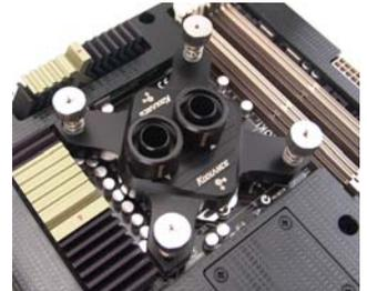
The CPU water block can be opened (for cleaning, etc.) by carefully unscrewing the four assembly screws with the included wrench. It is extremely important to reassemble this product properly. **WHEN REASSEMBLING, CAREFULLY HAND-TIGHTEN THE ASSEMBLY SCREWS AND DO NOT OVERTIGHTEN. IF DONE IMPROPERLY, THE ACETAL THREADS CAN BECOME STRIPPED OR CROSS-THREADED!**
