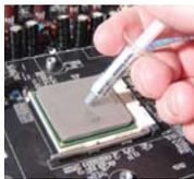
Apply thermal paste to the CPU directly. Spread the paste so that it evenly and thinly covers the CPU. A piece of thick paper (such as a business card) works well for this.
