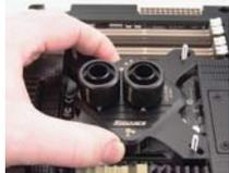
Place the water block over the mounting posts. The temperature sensor should already be installed on the cooler (if available).
