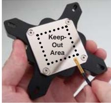
If a Koolance system is used, place the temperature sensor included with it on the edge or side of the water block's metal cold plate. *Make sure it is not covering any area that will be in contact with the CPU.*
