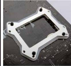
From beneath the CPU socket, carefully insert the back plate posts through the motherboard mounting holes. The insulating pad will be sandwiched between the back plate and motherboard.
