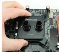
Place the water block over the mounting posts. The temperature sensor should already be installed on the cooler (if supported).
