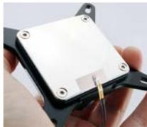
Trim out a piece of metal tape and apply it to keep the temperature probe in place. DO NOT stick metal tape or the temperature probe where the processor comes in contact with the cooler.
