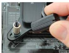
Over each mounting post above the top bracket, place a plastic washer, then a spring, and lastly a thumb nut. Tighten thumb nuts gradually in a cross-shape pattern. **DO NOT OVERTIGHTEN THUMB NUTS OR DAMAGE TO THE WATER BLOCK, PROCESSOR, OR MOTHERBOARD COULD RESULT!**
