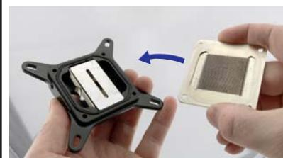
The cold plate microfins must run **perpendicular** to the impingement plate center slot!
