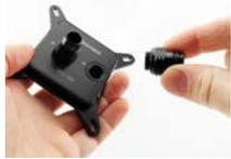
Install two G 1/4 BSPP threaded fittings (sold separately) into the cooling block. Hand tighten all fittings--overtightening can damage the block and threads.
