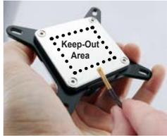
If a Koolance system is used, place the temperature sensor included with it on the edge or side of the water block's metal cold plate. *Make sure it is not covering any area that will be in contact with the CPU.*
