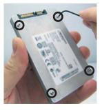
With the included hex wrench, install the threaded posts into the four mounting holes on the bottom of your hard drive.
