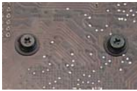
Typical heat sink screws
