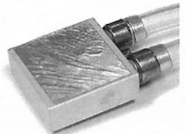
7) Peel both coverings off each side of the included thermal pad, and press against the videocard cooler. It should be attached metallic-side up, on the flat bottom side of the cooler (not the top side with the small central receptacle).
