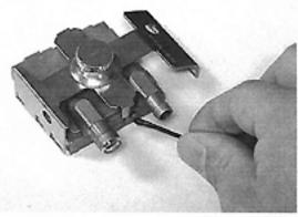
5) Insert the CPU thermal probe firmly into the special cavity (located behind the processor jacket). There is a thermal adhesive within the hole to help keep the probe there. We recommend zip-tying the probe wire to a nearby liquid tube for stability.
