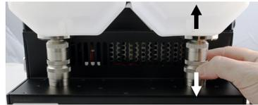
Consider labeling the containers once they are identified. Detach both from the RFS-500 by pulling down on the female fitting's lock ring.
