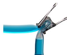
Hold "Refill" again until the loop and reservoir are adequately full. To avoid spillage from the reservoir fill port, it is safer to stop the RFS-500 early and complete coolant filling by hand.
