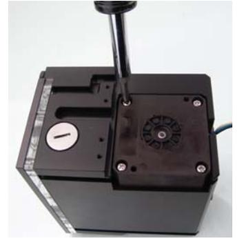
**NOTE:** If your pump version has feet on the plastic base, these must be removed in order to fit the RP-402X2.
