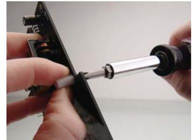
Make sure the connecting pins are aligned properly, and carefully insert the expansion board into the TMS main board.
