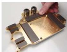
Place the 8 heat transfer pads on each additional area cooled by the Koolance liquid block. This includes 3 rows of memory, 4 power/VReg areas, and 1 PCI-Express controller chip.
