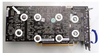
Example 2: 8800GTS Disassembly Screws
