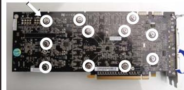
Example 1: 8800GTX Disassembly Screws
