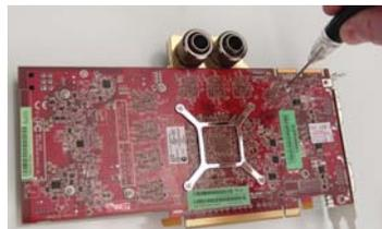
Koolance VID coolers include redundant G1/4 threading on both sides. This means the input/output nozzles can be placed on either side of the cooler.
