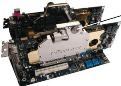
Two G1/4 "caps" are included with the VID coolers which can be placed opposite the desired nozzle locations.
