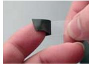
Thermal pads may have plastic film on *one or both sides* that must be removed before application.
