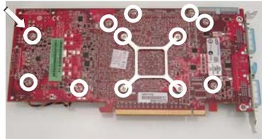
Example 2: HD 4850 Disassembly Screws
