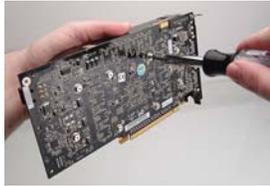
The spring-screws on the bottom side should be removed first. There should be 12-14 of these on the video card. There may also be smaller mounting screws on the side of the L-bracket.
