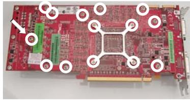
Example 1: HD 4870 Disassembly Screws
