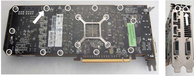
Radeon 290X Disassembly Screws (Bottom and Rear L-Bracket)
