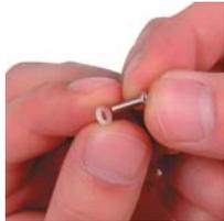
4 small mounting screws are included with the VID-AT1-V06. Thread an insulating washer onto each of these.
