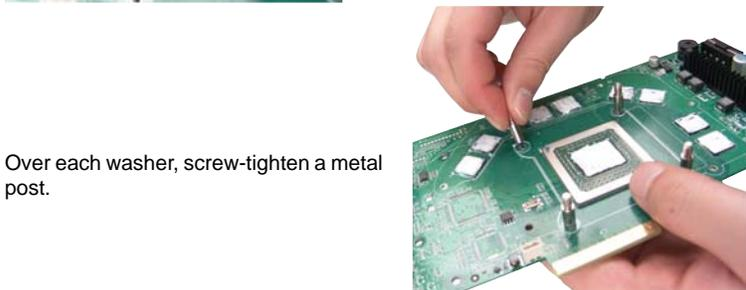
Over each washer, screw-tighten a metal post.
