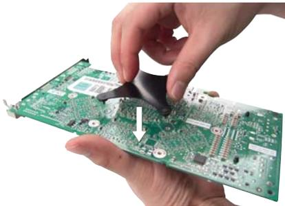
This piece aligns with the same 4 mounting holes as the original rear heat sink brace.
