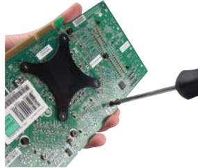
The mounting screws on the bottom side should be removed first. There may be 8 or more of these on your 6800 GT or Ultra card.
