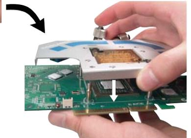
Finally, screw-tighten a mounting nut firmly to each metal post.
