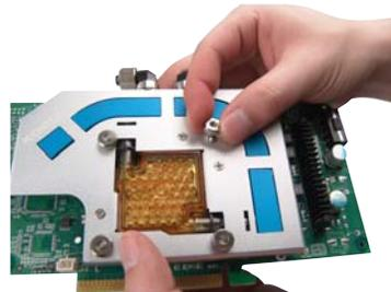
NOTE: Video card RAM chips are not perfectly flat with one another. To make sure your VID-NV1-L06 is making the best contact possible for your card, remove the cooler and examine the distribution of thermal paste.
