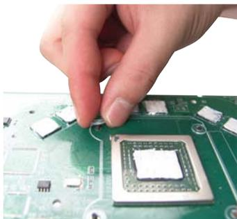
On front of the card, place plastic insulating washers on each of the 4 brace mounting screws.
