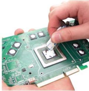
Additional thermal paste will likely be required on the GPU chipset and RAM modules after removing the original heat sinks.
