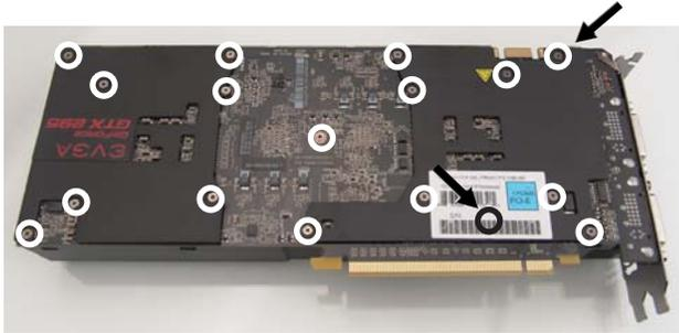
Remove both screws on the L-Bracket (if present).
