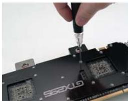
There are 17 screws. 14 thread into the front water block. The remaining 3 are threaded into the included Koolance metal pegs shown below:
