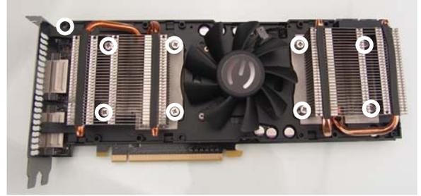
The heat sink and fan can now be **carefully** removed from the video board. All original thermal paste and padding should be cleaned off the card. Replacements are provided with the Koolance water block.
