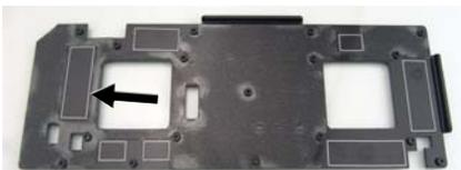
2 With a flat screwdriver, depress the locking tabs around the edges of the heat sink to release its cover.
