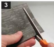
The thermal pad sheet should be cut into pieces required for your video block contact areas. Please use the diagram included with your water block to determine the approximate sizes that will be needed.
