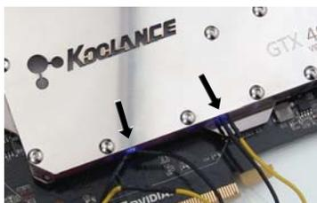
The included LED cable can be optionally installed into the bottom edge of the VID-NX460. It will connect to the video card's fan header.
