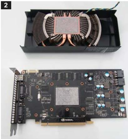
**Carefully** remove the heat sink. Original thermal paste may present resistance during removal.
