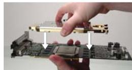
Place the Koolance block onto the video card so the mounting screws will align.
