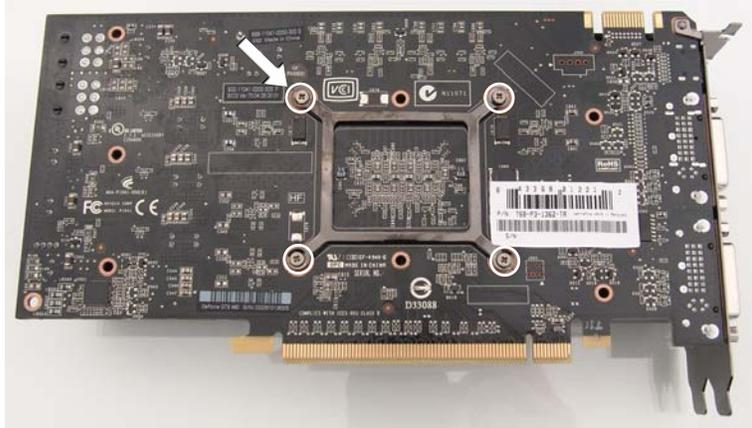
GTX 460 Disassembly Screws
