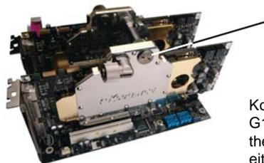
Two G1/4 "plugs" are included with the VID coolers which can be placed opposite the desired nozzle locations.
