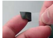
Gray thermal pads have plastic film on *both sides* that must be removed before application. White/Pink thermal pads only have plastic film on *one side* (white) that must be removed. Do this after cutting the proper shapes.
