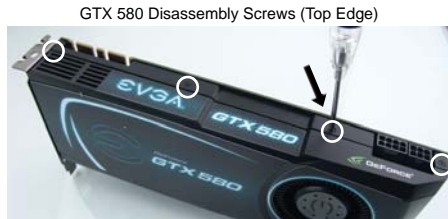
GTX 580 Disassembly Screws (Top Edge)
