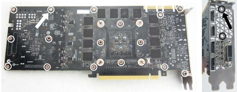
Titan X Disassembly Screws (Bottom and Rear L-Bracket)
