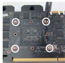
Optional Koolance Back Plate Thermal Pad Locations
