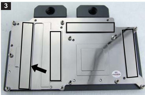
VID-NXTTNX Water Block Thermal Pad Locations
