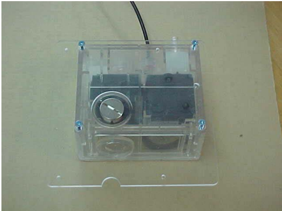
Place the Adapter over the bottom of the reservoir, and insert 4 silver screws as illustrated above. (bottom view)
