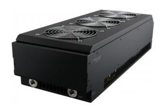
HXM-ALX2000 is a triple fan heat exchanger for Koolance's <u>ALX modular cooling systems</u>. When combined with an <u>RPM reservoir and pump module</u> (sold separately), the heat dissipation is approximately 2000W. Front fitting threads are G 1/4 BSPP, and the rear are 1/4 NPT.
