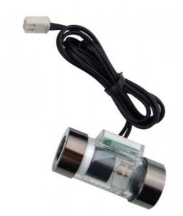
Koolance's inline flow meters provide electronic indication of real-time coolant flow rate. This model uses a reed switch to detect impeller rotation. G 1/4 BSPP fitting threads, and primary materials are nickel-plated brass and acrylic. Approximate read range is 1.0-20 LPM (15.6-317 GPH). Wire length is about 28" (70cm). It is recommended to keep current through the flow meter at 10mA or less to prevent damage.
