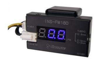
INS-FM18D combines an LCD display with Koolance's stainless steel flow meter in a small footprint. The display shows flow rate in liters per minute (LPM) only. A 12VDC connection is required for power. Primary materials are a stainless steel body with nickel-plated brass G 1/4 BSPP threads.
