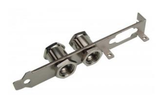
Dual panel-mounted socket threads for "internal/external" fittings on a computer chassis L-bracket. The female G 1/4 BSPP threaded couplings can be removed from the L-bracket and used as panel-mountable unions. Nickel-plated brass. This product may need to be temporarily disassembled during installation.
