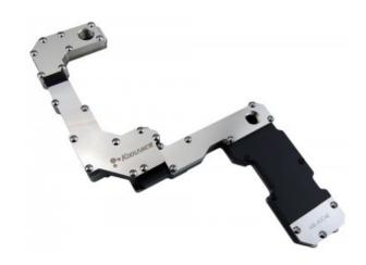
The MB-ASC4E water block is designed exclusively for the ASUS Crosshair IV Extreme motherboard. It liquid cools the northbridge chipset and other nearby components. Materials include copper with anti-corrosive nickel plating, acetal body, and steel top cover. G 1/4 BSPP fitting threading.
