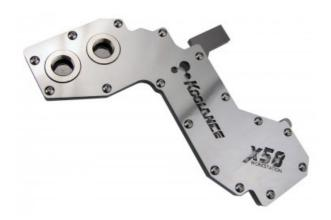
The MB-ASP6WR water block is designed exclusively for the ASUS P6T6 WS Revolution motherboard. It liquid cools the northbridge and southbridge chipsets, along with nearby components. Materials include copper with anti-corrosive nickel plating and an acrylic top. G 1/4 BSPP fitting threading.
