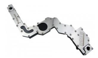
The MB-ASR3E water block is designed exclusively for the ASUS Rampage III Extreme motherboard (not included). It liquid cools the northbridge chipset and other nearby components. Materials include copper with anti-corrosive nickel plating, acetal body, and an acrylic and steel top cover. G 1/4 BSPP fitting threading.
