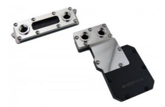
(Motherboard and CPU block are not included.) The MB-ASSTX79 water block is designed exclusively for the ASUS Sabertooth X79 motherboard. It includes two custom water blocks for the primary chipset and VRM. Materials are copper with anti-corrosive nickel plating, and an acetal body. G 1/4 BSPP fitting threading.
