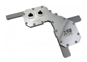
The MB-EVX58CF water block is designed exclusively for the EVGA X58 Classified motherboard (141-BL-E759-A1 and 141-BL-E760). It liquid cools the northbridge and southbridge chipsets, along with nearby components. Materials include copper with anti-corrosive nickel plating and an acrylic top. G 1/4 BSPP fitting threading.
