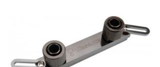
The MVR-100 is a universal water block for motherboard MOSFET-based voltage regulator circuits. Koolance offers various swappable cold plates for the MVR-100 to fit a wide variety of motherboard brands and models. Materials include copper with anti-corrosive nickel plating. G 1/4 BSPP fitting threading.
