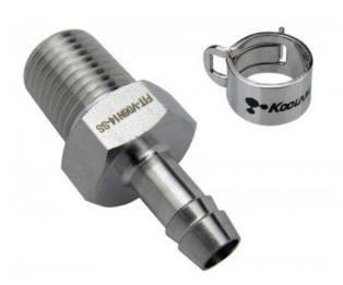
Single hose barb fitting for 1/4in (6mm) ID tubing. 1/4 NPT (tapered) thread. Includes hose clamp for 3/8in (10mm) OD tubing.
