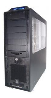
Get the maximum amount of space for large single or dual CPU systems with the PC3-736, which provides support for motherboards up to  $12" \times 13" (30.5 \text{cm} \times 33 \text{cm})$ .
