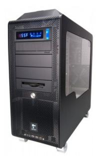
What does it take to reach 1000W of heat dissipation? The PC4-1000 series provides the first 1kW liquid cooling solution by Koolance. In this new generation, performance is accelerated with over three times the coolant flow rate of previous dual-pump systems (8.5 L/min, 2.25 GPM), a triple 120mm fan heat exchanger, and updated electronics.
