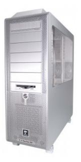
The PC5-1300 series offers heat dissipation of up to 1300W using a Koolance pre-installed quad-120mm fan heat exchanger. There is no pump included with this system, allowing you to choose among Koolance's <u>RP-1000</u>, <u>PMP-450</u>, <u>PMP-400</u>, or anything else! (Note: The RP-1000 is the reservoir, pump, and electronic control unit used in the Koolance PC4-1000 series system.)
