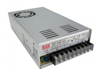
This is a power supply and wiring kit to power the Koolance EXC-450 or VLX-450 chillers from an AC outlet. DC and AC wires are included (AC plug is for North American outlets). The power supply is auto-switching, 100-240VAC 50/60Hz input to 24VDC output. It is rated to 312W, with PFC, and is CE and UL labeled. The size is approximately 9in x 4.5in x 2in (230mm x 115mm x 50mm).
