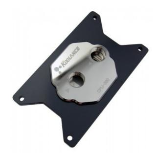
Koolance's CPU-390 redefines thermal performance again with an all-new 0.17mm microfin process and internal flow optimizations. Versions are available with acrylic and copper tops.
