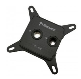
Koolance's CPU-400 features record-breaking thermal performance with a microfin nickel-plated copper cold plate, acetal top, and rugged steel mounting bracket. Standard G 1/4 BSPP threading will accept any Koolance fitting diameter up to 19mm (3/4in) OD compression style. Please select the desired fitting type for this base model (it does not include fittings). The CPU-400I supports most boards using the following processors:
