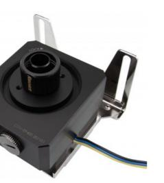
COV-RP400 is an acetal fitting and reservoir base for the Koolance PMP-400 pump. Pump, reservoir, and fittings are sold separately. Along with enabling the use of any G 1/4 BSPP (parallel) thread fitting style and diameter, it allows flow to be specifically directed for increased pump performance or broader chassis integration. Fitting base, mounting bracket, coupler for 60mm OD reservoirs, socket plug, and mounting hardware is included.
